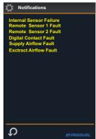
Supply / Extract Airflow Fault; if in HOME/BOOST modes and either Al1 or Al2 is reading less than the Airflow Alarm limit value after the alarm delay parameter (0..60 mins), the airflow alarm is raised.
