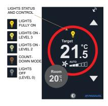
When the Lights icon is pressed the device goes to COUNTDOWN mode for the time set in the Lights Delay Time parameter. In this mode the Lights icon changes colour to brown. If the Lights icon is re-pressed in this mode the countdown is cancelled and the lights are switched back to fully ON level.
