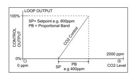
output starts to modulate to 100%. When the CO2 level is the amount of the Proportional Band above the setpoint, the loop output is 100%. The configuration is done via the configuration parameters. The CO2 control loop can also be configured to operate as Proportional + Integral control by changing the Integral Action Time from 0 to a required value. The actuator direction can be changed via Output Direction parameter (Direct, Reverse).
