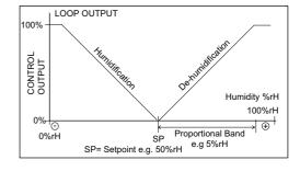
In the ECO mode the humidity output is set to 0%.
