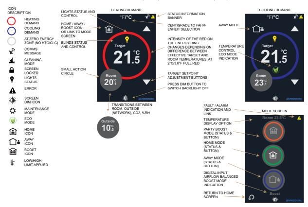
The colour of the 'Energy Ring' indicates the heating/cooling demand. The 'Energy Ring' is white at 'deadzone'. The density of red/blue on the 'Energy Ring' modulates based on how far from the
