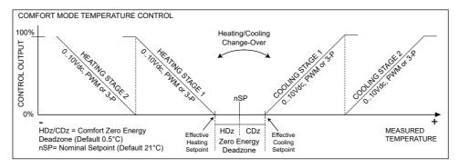
Between heating and cooling stage 1 is a 'deadzone'. With P-control in the 'deadzone' the cooling and heating loop demand is 0%. With PI-control, if the temperature remains in the 'deadzone' for a prolonged period, the heating/cooling demand ramps to 0%. The 'deadzone' allows the temperature to fluctuate around the setpoint without heating or cooling valves starting to open. The TRC-A-3A has a built-in lock that prevents cooling and heating demands to be on simultaneously.
